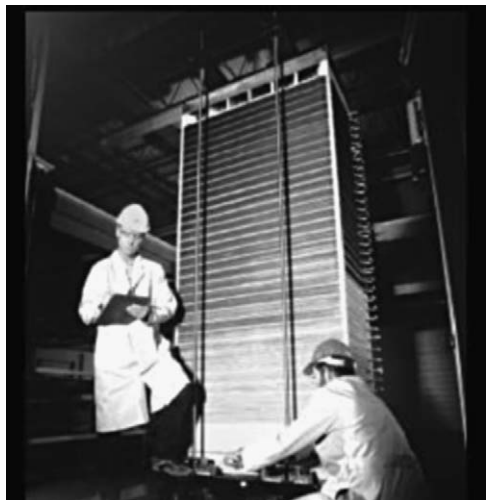
Fig. 8. Full-size stack completed at the FCE manufacturing facility: ~350–400 cell stack.
